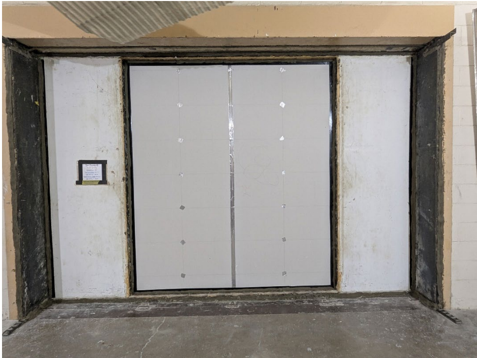
Figure 2 – Specimen mounted in test aperture, as viewed from receive
